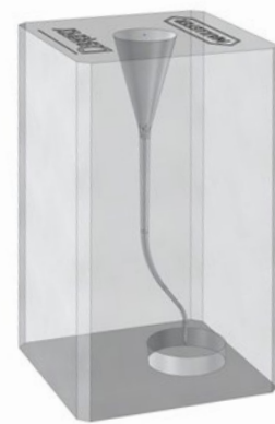
Figure 2: Number of “S”-shaped canals (picture on the right) treated before unwinding could be detected by visual inspection. ProTaper Ultimate™ shows higher unwinding resistance compared to all competitor files, n=5 per group (6). Brasseler EndoSequence CM Taper Files, Komet F360, FKG Race Evo, Edge Taper Platinum are not registered trademarks from Dentsply Sirona.
